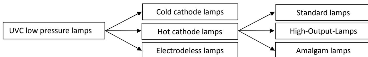
Except the cold cathode lamps we are able to produce all types in our own fabrication including characteristic customization.
