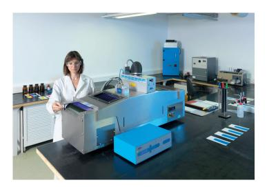
To ensure the highest quality, all UV lamps are measured in irradiation chambers or specially equipped dark rooms before they leave our premises.
